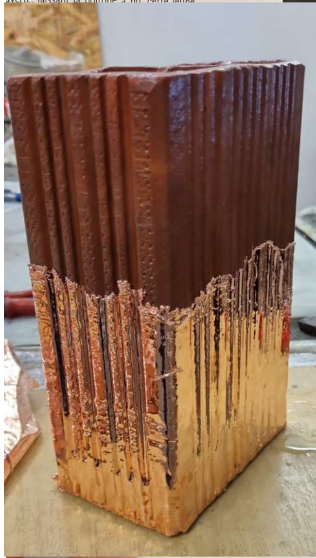
Serena experiment / Brick with copper galvanisation
